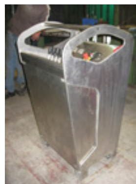
Early stages, with aluminium cut and shaped to fit the design.
